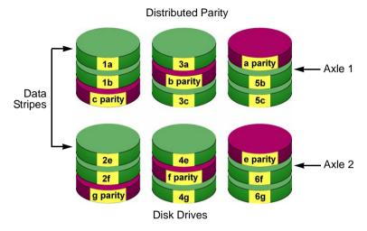
Figure 5. RAID 50 Striping of Distributed Parity disk arrays
